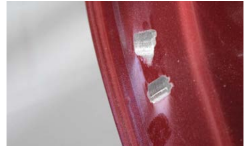
Spot-weld has been ground just enough to remove the top layer of the nugget and not damage the bottom panel.
