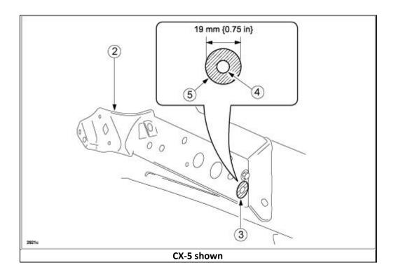
**NOTE:** After installing the bolt (4), apply touch-up paint to the exposed base material area of the front fender stay.
