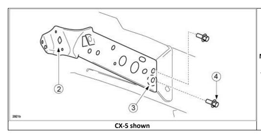
**NOTE:** Do not paint ground point (3) where attachment bolt (4) is seated.
