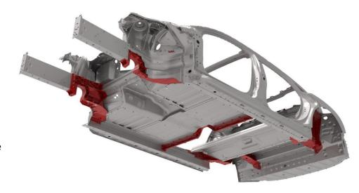
Non-serviceable casting components are critical to the overall structural integrity of our products. Any unauthorized repairs performed on non-serviceable parts is likely to impair the structural integrity of the non-serviceable part and negatively impact safety
