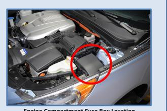
**Engine Compartment Fuse Box Location**
