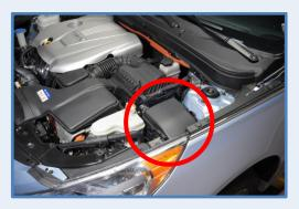
3. Remove the IG1 relay (tan). Refer to the illustration for relay location.
