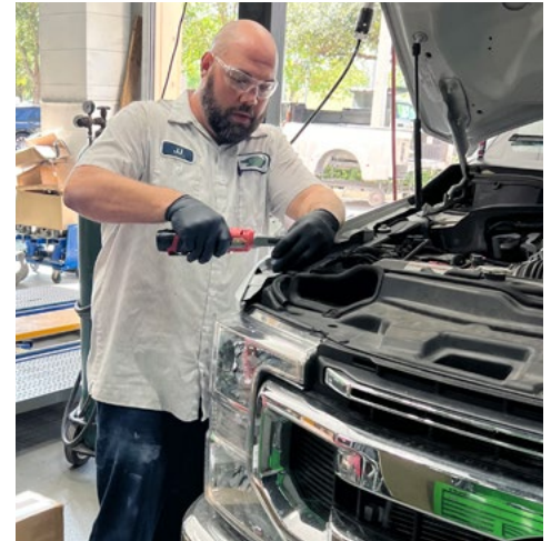
Repair technician JJ Mills removes a headlight in preparation for refinishing the right side of the cab and fender after replacing the door and cab corner.
